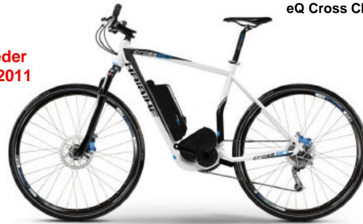
Rahmen: Aluminium 6061, hydroforced tubes Gabel: Rock Shox Reba SL,
